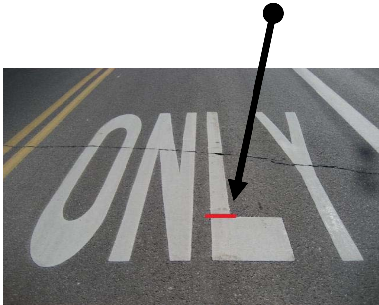
Figure 7. Placement of Retroreflectometer on L Location
