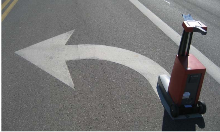
Figure 6. LTL-X Retroreflectometer on Arrow Location
