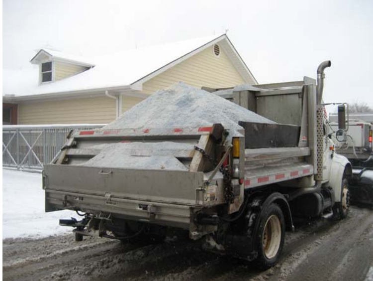
Figure 9. Salt/Limestone Grit in Bed of Plow Truck
